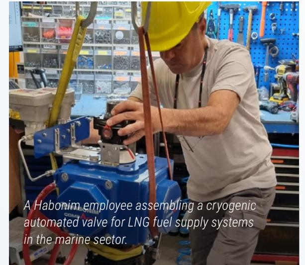
*A Habonim employee assembling a cryogenic automated valve for LNG fuel supply systems in the marine sector.*
