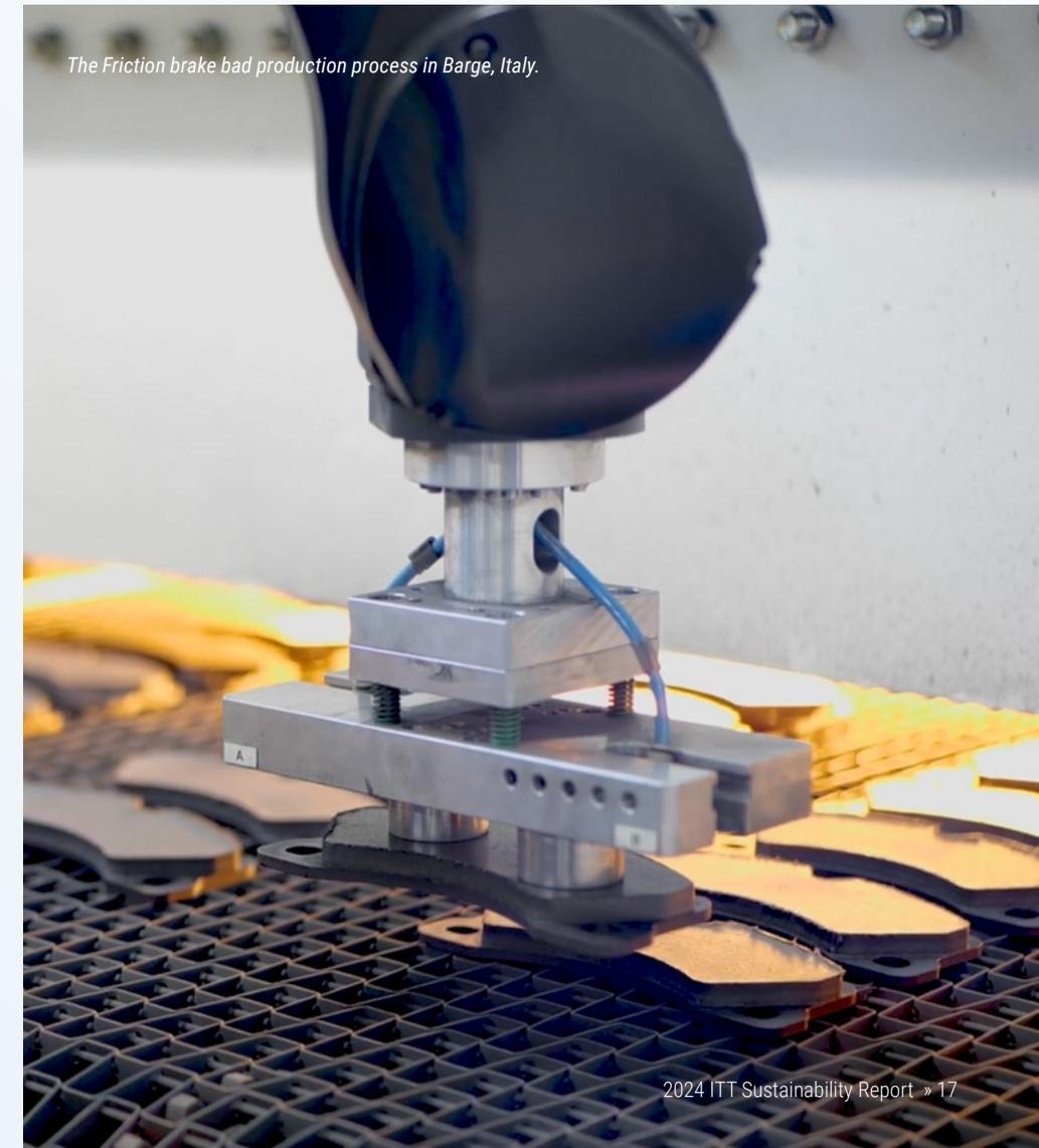
*The Friction brake pad production process in Barge, Italy.*
