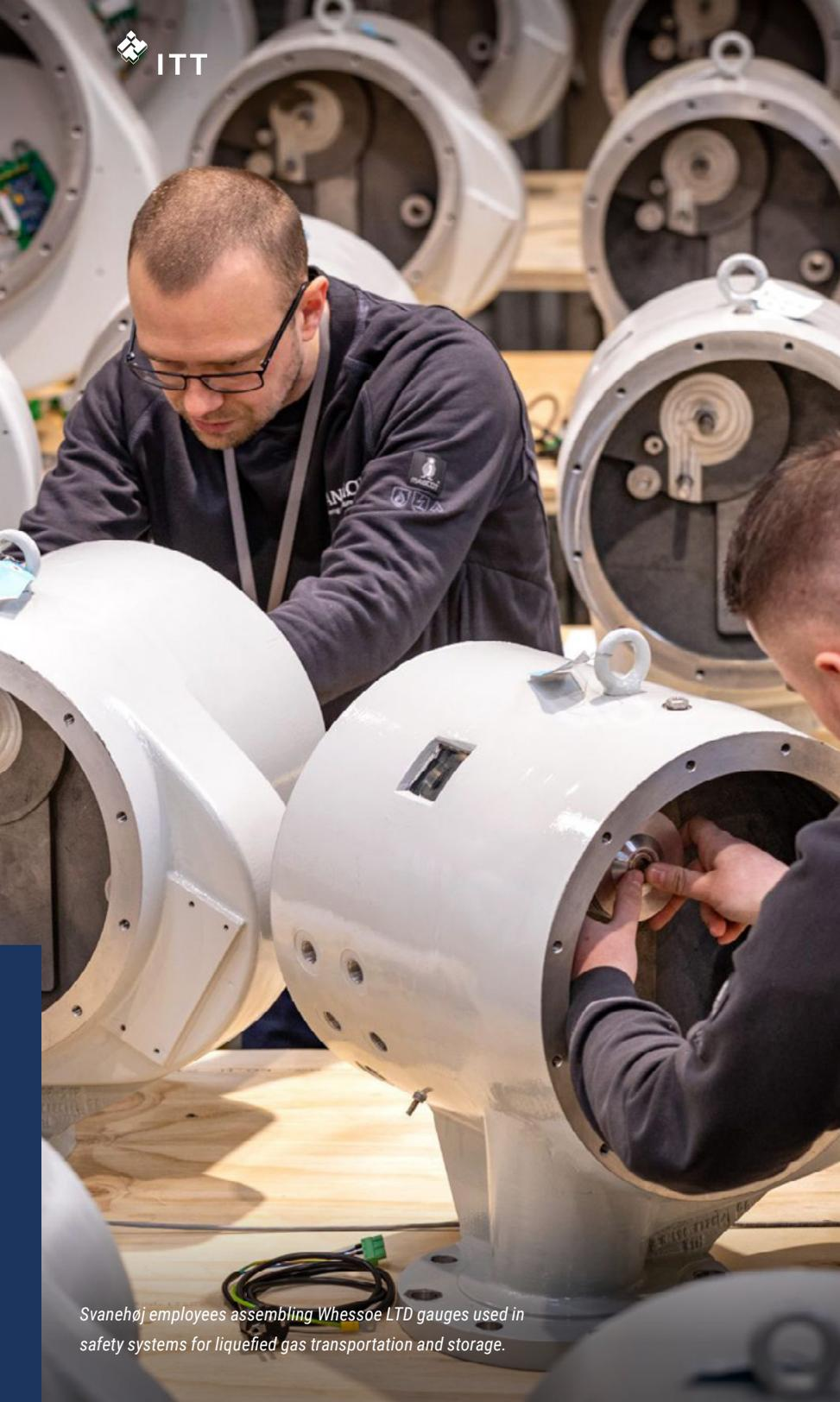
Svanehøj employees assembling Whessøe LTD gauges used in safety systems for liquefied gas transportation and storage.
